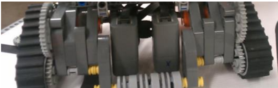
The parts of the robot which held the wheels were attached to each other so the wheels would not bend inwards.
