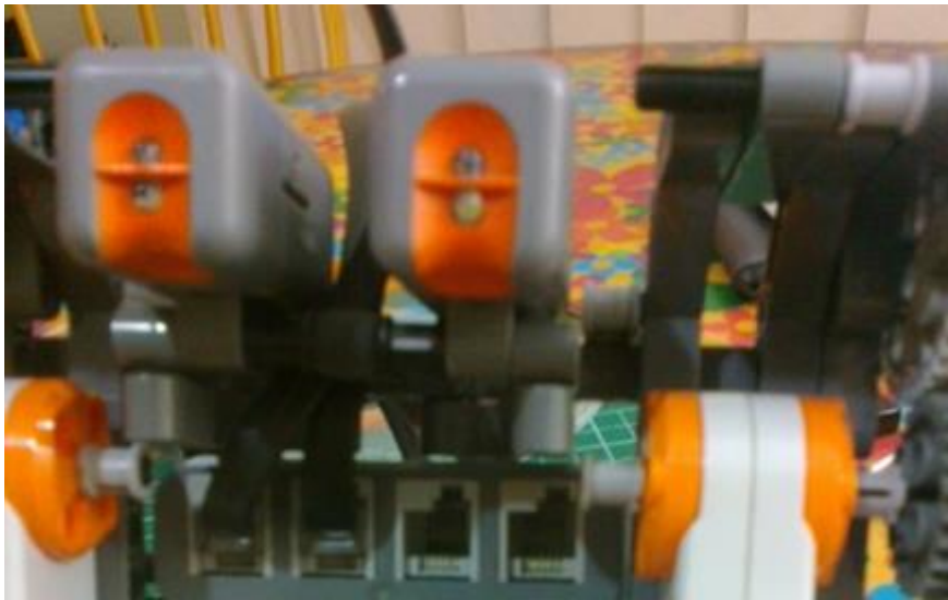
The light sensors were placed close to each other for better line following.
